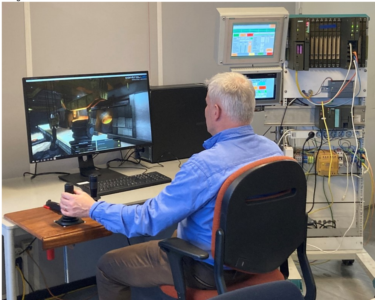
Figure 5 - HIL-test charging crane in action
