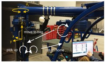
The first simulations showed that the motion was not optimal. The robot arms were moving in such a way that the individual motors were overloaded. A better motion strategy could reduce the individual motor loads significantly.
