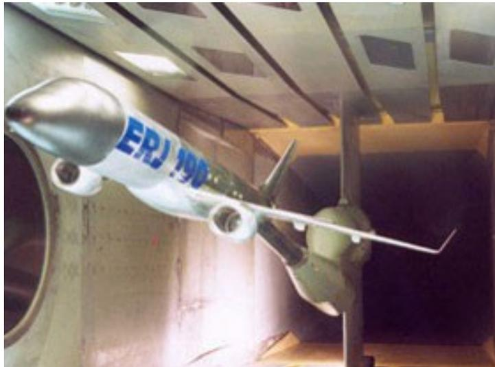
In Amsterdam DNW operates a high speed wind tunnel. In this tunnel an area of 2.0 m x 1.8 m is available for testing from mach ranges of 0.1 up to 1.35 and pressures ranging from 0.2 bar to 4.0 bar. A robot is used to maneuver models into the test area and keep them in the correct postures.
