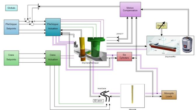
The best way to analyze dynamic systems is by using 3D simulation models. Such a simulation model will describe the motions and forces of all the components in 3 dimensions (3 translations and 3 rotations).
