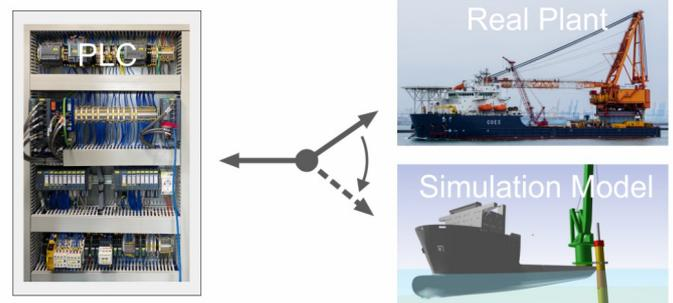
With HIL simulation you can also test the control software for a pile gripper under conditions that are impossible or dangerous with a real gripper. This allows you to verify the correct operation of your code to a degree impossible otherwise.
