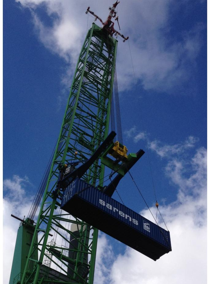
container and then upgraded to a wind blade. The tag lines could stabilize the wind blade in wind speeds up to 15 m/s. Since 2015 the system is in full operation and used for hoisting wind blade, nacelles and other loads.
