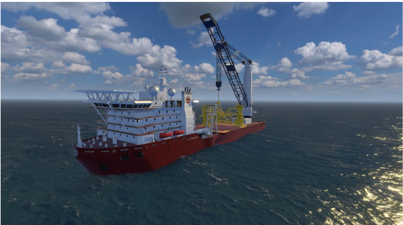
Figure 1: Heavy lift vessel with crane and template.
