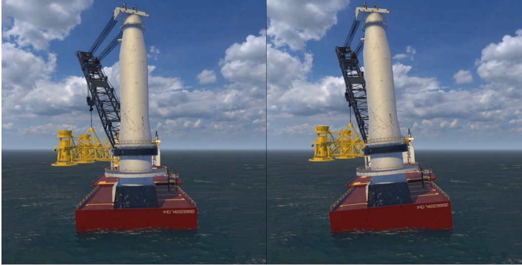
Figure 17: Offloading with and without ballasting.
